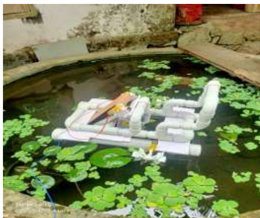
Fig 9.2 the testing of oil skimmer
