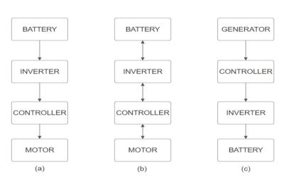
Diagram (a) shows how the battery powers the motor when the car is in electric mode and not using brakes.
