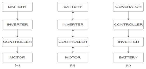
Diagram (a) shows how the battery powers the motor when the car is in electric mode and not using brakes.
