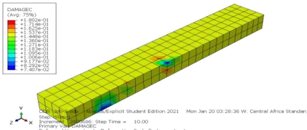
Figure 11: Post processing result for the compression damage using the Hognestad Model
