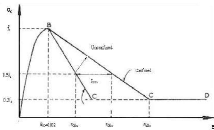
Figure 2: Uniaxial Compression curve for Kent and Park Model
