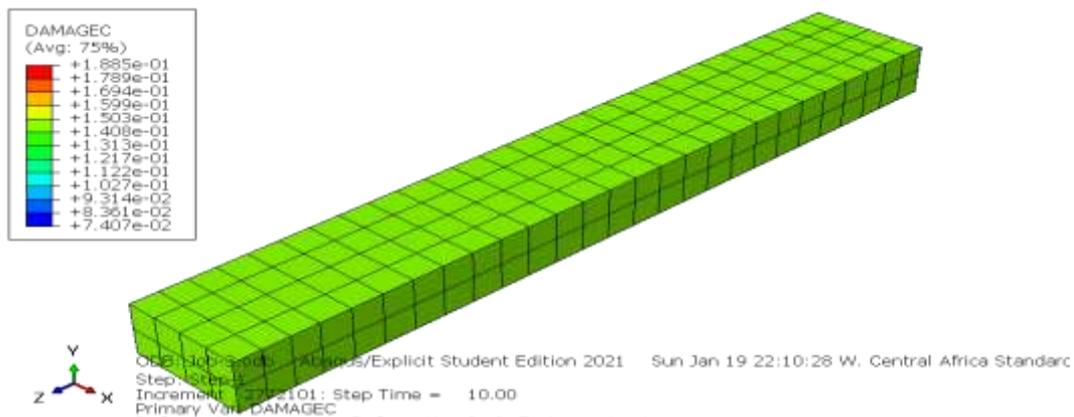
Figure 13: Post processing result for the compression damage using the Kent and Park Model.
