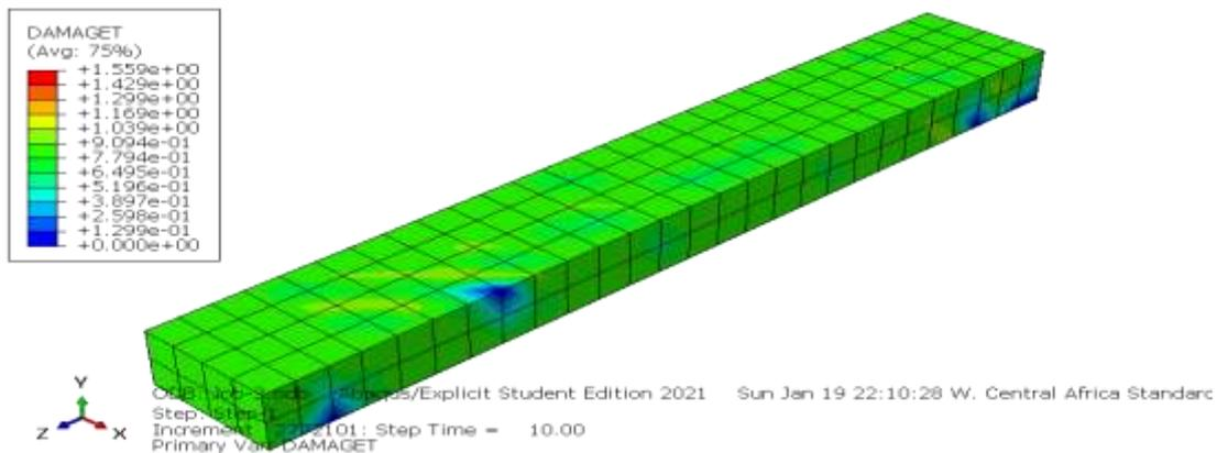
Figure 12: Post processing result for the tension damage using Kent and park model
