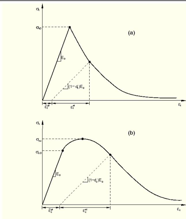
**Figure 1:** Response of concrete to uniaxial loading in tension (a) and compression (b).
