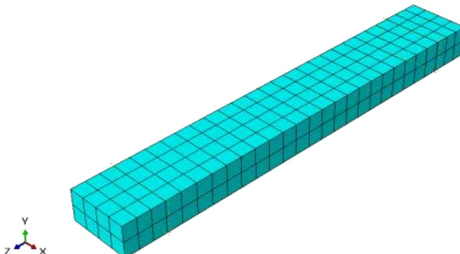
Figure 9: Mesh System with Hex element for the 150mm Beam model.
