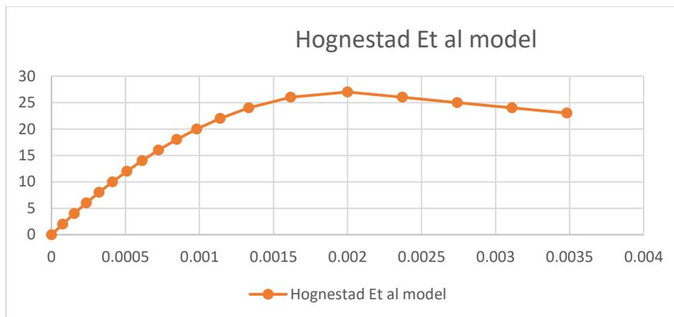
**Figure 5:** Stress-Strain curve Hognestad et al model
