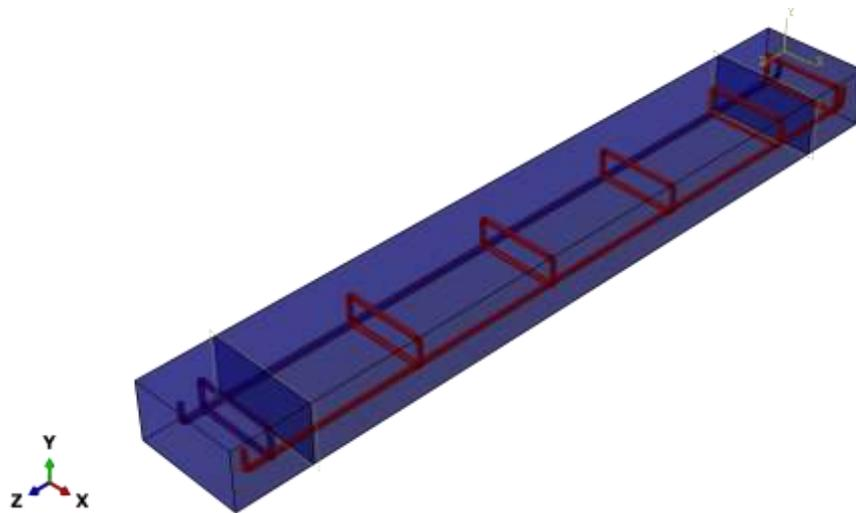
Figure 8: reinforcement bars embedded in the 150mm concrete Beam
