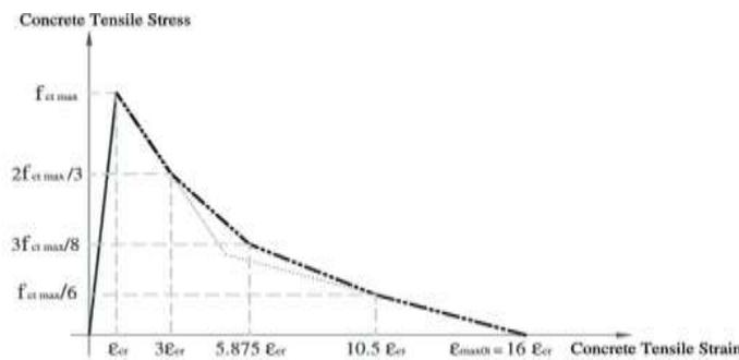
**Figure 6:** Concrete tensile stress strain curve by Said and Mohie, 2012
