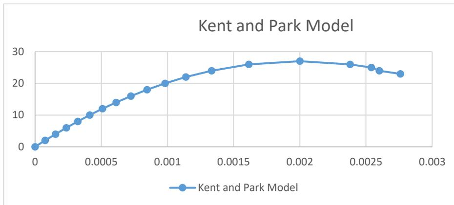
**Figure 4:** Stress-Strain curve. Kent and Park model
