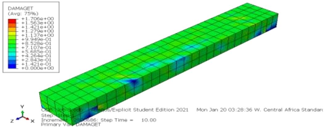
Figure 10: Post processing result for the tension damage using the Hognestad model
