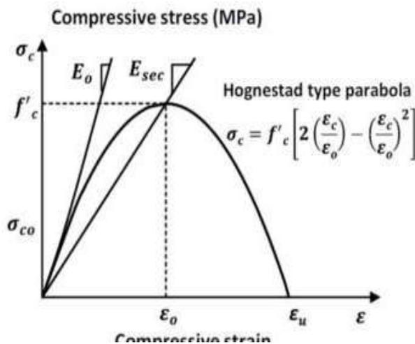
Figure 3: Uniaxial Compression curve for the Hognestad et al Model
