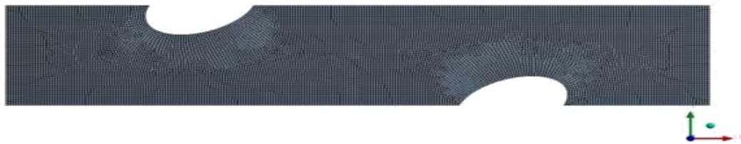
Figure 4.: Meshing of plate fin with elliptical tube inclined at 30° heat exchanger
