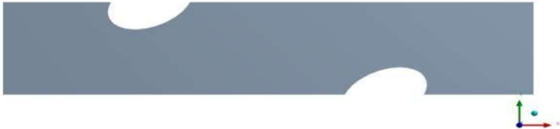
Figure 3: CAD model of plate fin with elliptical tube inclined at 30° heat exchanger
