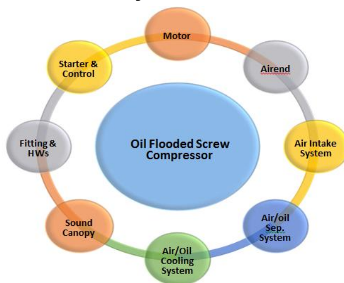
Fig.2. Schematic depiction of the components of an oil-flooded rotary screw compressor
