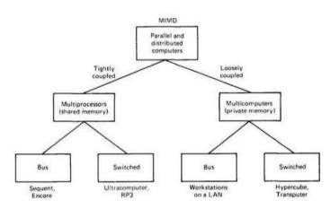
Although all distributed systems contain multiple processors, there are many alternative ways to combine them, and as Flynn (1972) knew 2 basic characteristics of to classify portable multiprocessor systems: the number of instruction streams and therefore the amplitude of the knowledge flow.
