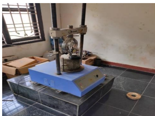
Fig:2 California Bearing Ratio Test Apparatus
