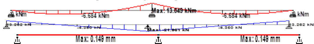
Bending moment, shear force and displacement diagram for poststress beam
