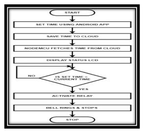
Step 1: Set the timing according to schedule with the help of android application.
