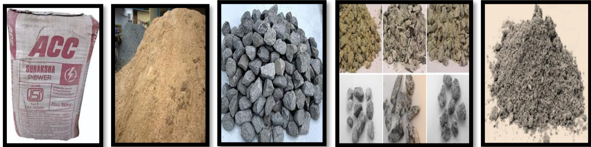
Figure 3 Cement, Fine Aggregate, Coarse Aggregate, Crushed Rock Sand, Volcano Ash
