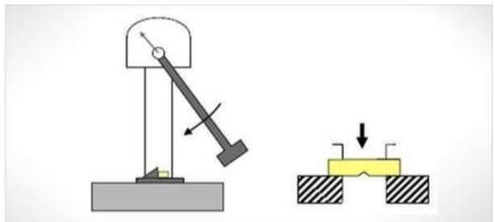
Presto assembles and supplies a wide range of **Plastic testing Instruments**. Out of the available range of testing machines, one of the widely used testing devices to test the impact tolerance / resistance strength of plastic is charpy impact test.
