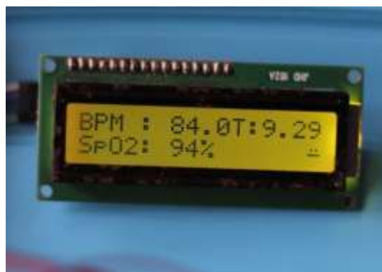
Figure 3: LCD displaying the real time output from sensors
