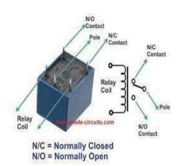
A relay is an electrically operated switch. It consists of a set of input terminals for a single or multiple control signals, and a set of operating contact terminals. The switch may have any number of contacts in multiple contact forms, such as make contacts, break contacts, or combinations thereof
