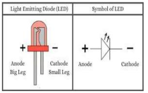
When an electric current passes through a semiconductor device called a light-emitting diode (LED), the LED emits light. When current flows through an LED, the electrons and holes recombine and produce light. LEDs only let current flow in one direction—forward—and stop it from going the other way.
