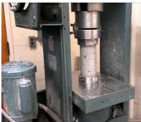
Fig. 3 Cylinder testing in compression testing machine.
