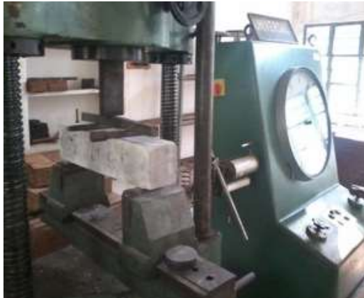
Fig. 5 Beam testing in Flexural testing machine
