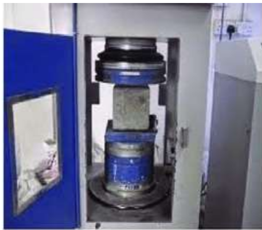
Fig. 1 Cube testing in compression testing machine
