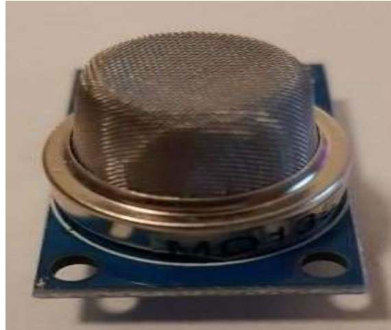
Fig 6: A MQ135 sensor on a small PCB.
