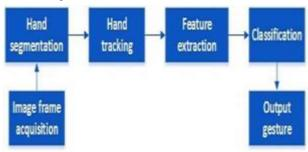
The technique that is used to recognize hand gesture is basis on computer vision. The overall system architecture is shown in figure 3 above. The whole system of hand gesture recognition divided into four phases: Image Acquisition, Image Pre-processing, Feature Extractions and Hand Gestures Recognition. Reading the video, Frame extraction and Pre-processing comes under the first stage i.e., video acquisition module
