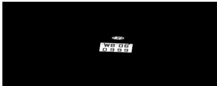
Figure: 4.3 -Problem in distinguishing the actual plate position due to light.
