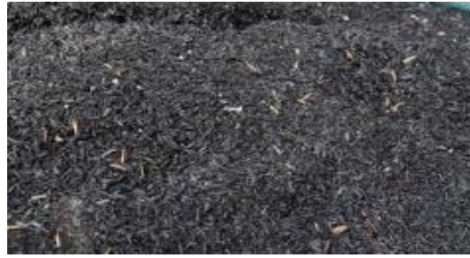
Fig.3.5 open burning technique was used to transform rice husk into ash at temperatures that vary from 3000C to 4500C (Stage-II).
