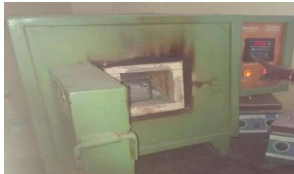
Fig. 3.6 The residual ash from the burned husk was subjected to further combustion at a temperature of 6500C for a duration of 2 hours (Stage-III).
