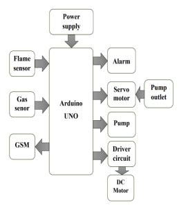
The autonomous firefighting robot which is an integrated system has more features. In this project flame and gas sensors were used for continuous monitoring to detect the fire and smoke. Once the fire/gas detected, the sensors alert the microcontroller and the controller starts alarm sound and an alert message which will be given to the registered mobile number through GSM.
