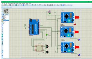
The above figure shows the detection of flame by glowing of the LED, it means the system has started and starts moving to extinguish the fire.
