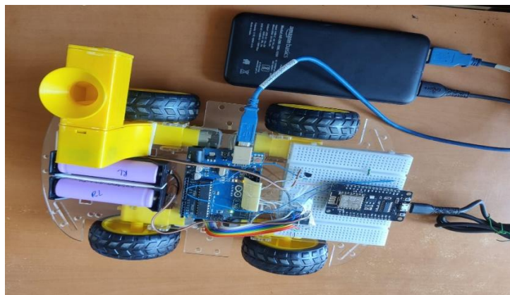
Fig: 3 CHASSIS CONNECTED WITH ARDUINO BOARD AND ESP CONTROLLER
