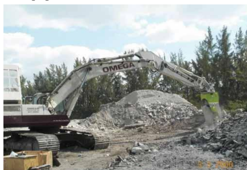
Fig 1.3 Long Boom Arm Hydraulic Crusher
