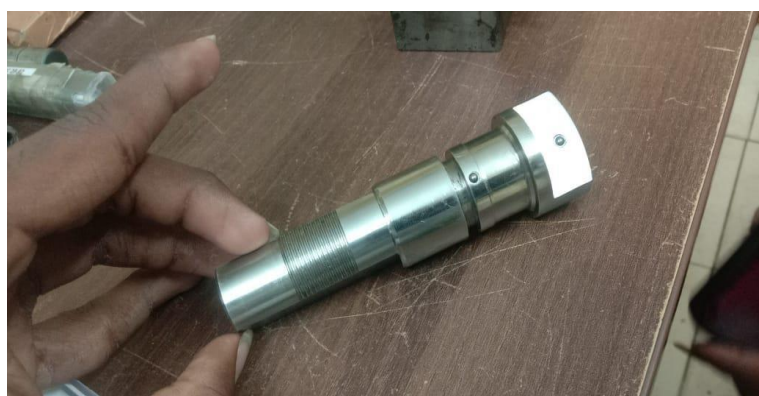
Figure 4: Finished Component (Drilled holes of 2 different diameters)
