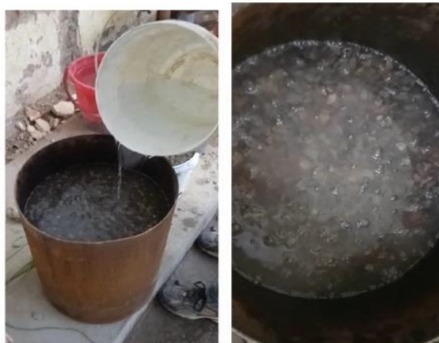
Fig. 5.1 Using a mild acid to treat CRCA.
