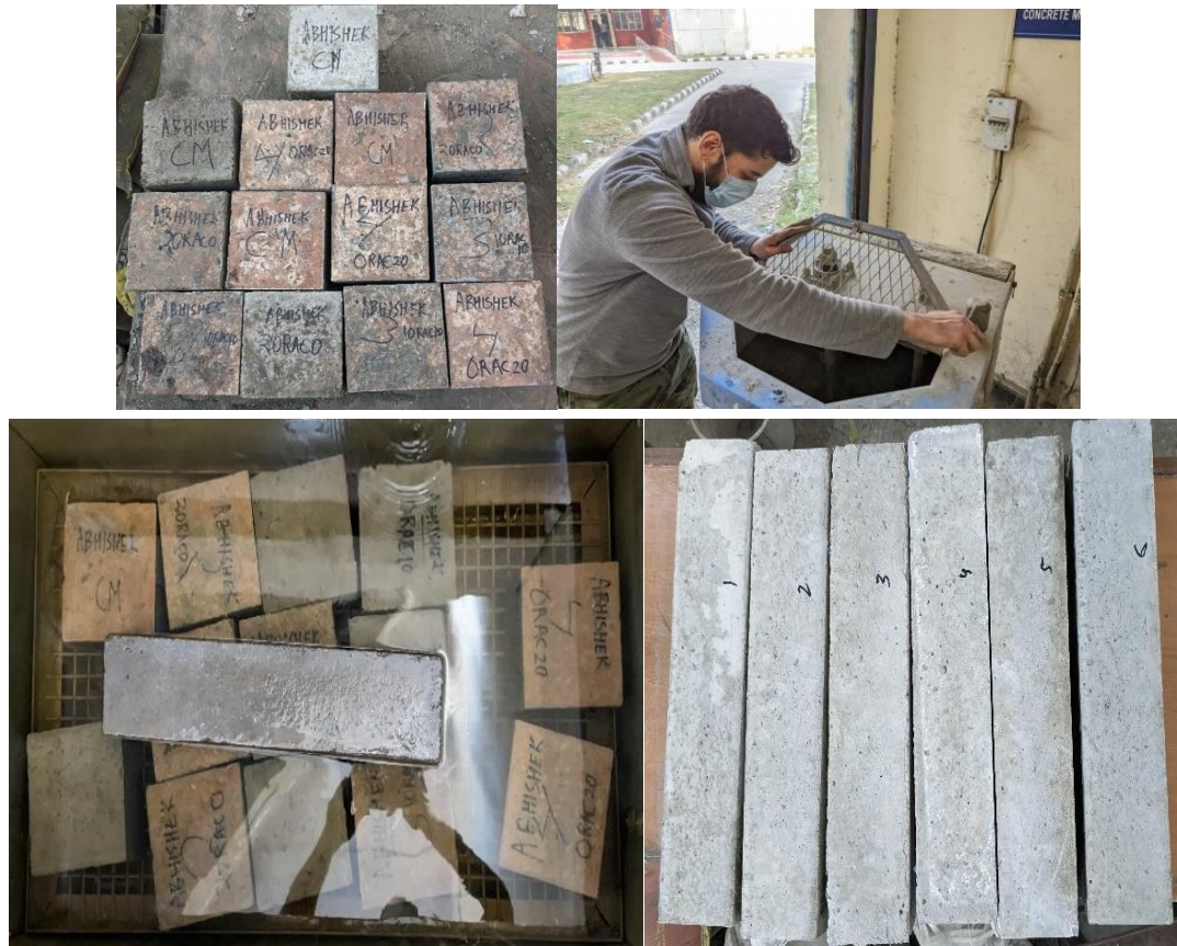
Fig. 4.4 (a) Mixing of concrete in mixer; (b) A batch of samples made for compression testing; (c) Curing of samples; (d) Samples made for Flexure testing.
