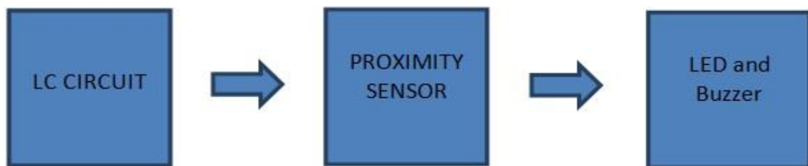
Fig No: 3 Block Diagram of Metal Detector
