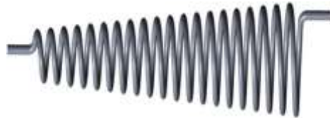
Fig 1. Cone helically coiled tube
