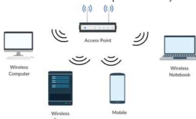
Figure 3. The 802.11 network Infrastructure operating modes
