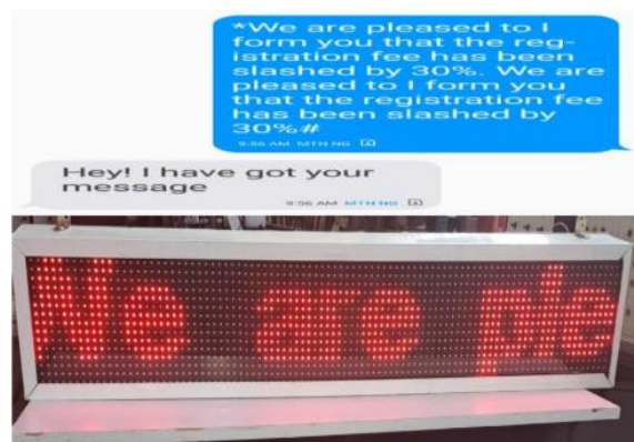
Fig.6: Displaying of the 160 character sent to the billboard display
