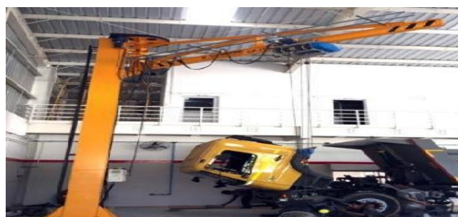
Figure 1: Fabricated Floor mounted jib crane [4]
